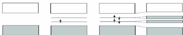
Figure 1. Diagram of evolution of the bands during the doping process by introduction of positive ions
