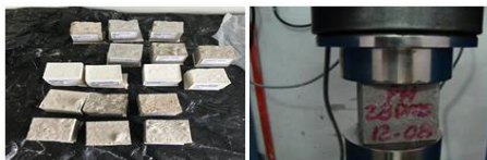
Figure 2. Samples and compression test method for mortars.
