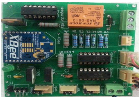
Fig. 8. Signal conditioning board.
