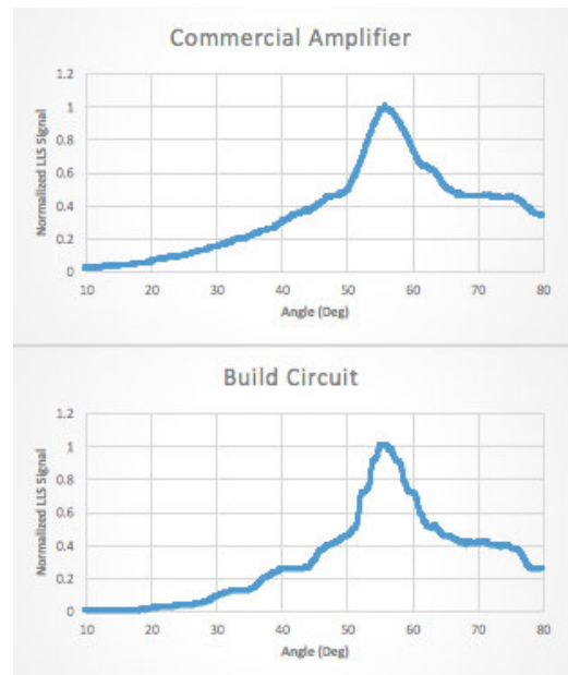
Fig. 10. Plot comparative between (a) built circuit and (b) comercial lock in.
