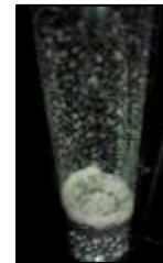
Fig. 2) Cohesive Powders tend to stick to walls and agglomerate.
