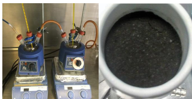
Figure 6. Laboratory synthesis equipment and wet FeS 2 .
