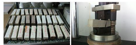
Figure 1. Samples and bending test method for mortars.
