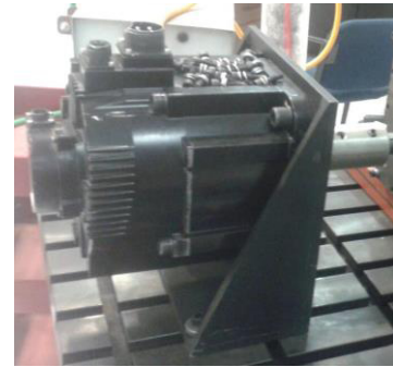
Fig 4. Motor SGMGV-44A3A6C model.
