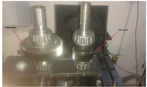
Fig 7. Entry gear and output gear.
