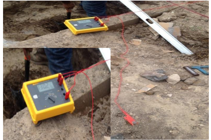
Figure 3. Colocation of Fluke device for measuring the resistivity of the natural ground and subsequent measurement of such resistivity.
