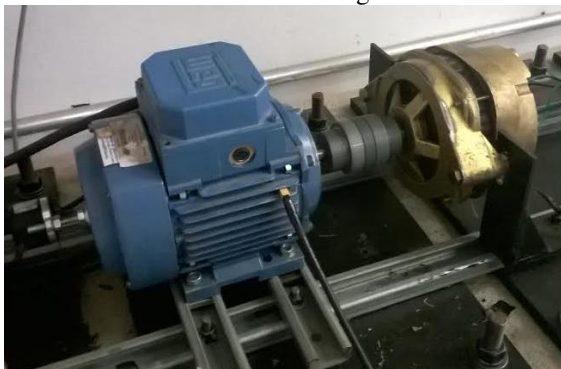
Fig. 6. Induction motor on the test rig.
