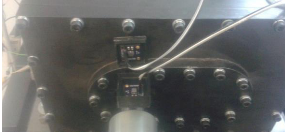
Fig 5. Radial and axial accelerometers.
