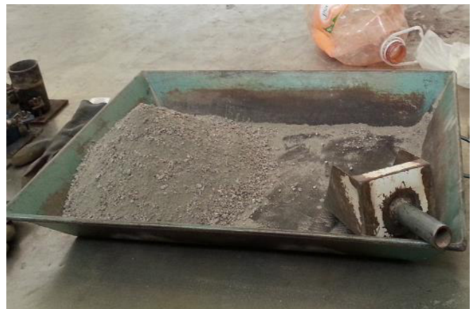
Fig. 1. Homogenizing of dry materials.
