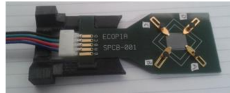
Figure 5. 4-way sample holder brand bridge technologies model SPCB-1 with 3D printed support.
