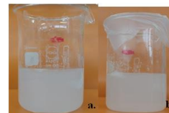
Figure 3 Solutions of nanoparticles of CS/TPP/LA, a). 0.2% CS/TPP 2ml LA, b) 0.2%CS/TPP 4ml LA.
