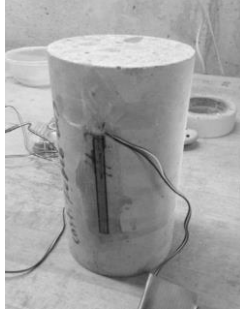
Fig 3 Concrete cylinder, f'c = 250 \text{ kg/cm}^2 , and a FBG sensor attached to the body of the cylinder for its further analysis.
