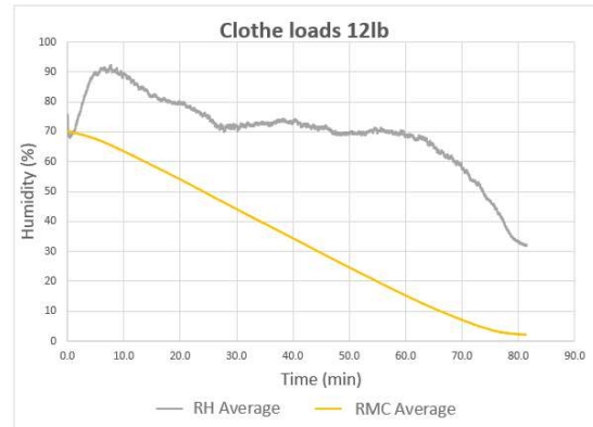
Fig. 3. Trend of Humidity RH average and RMC average during a drying cycle for a load of 12 lb.
