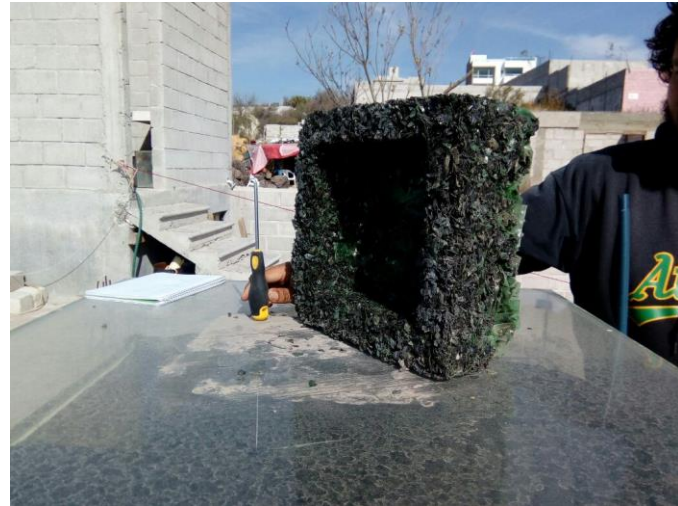
Figure 2.0 Cassette prototype made with PET.
