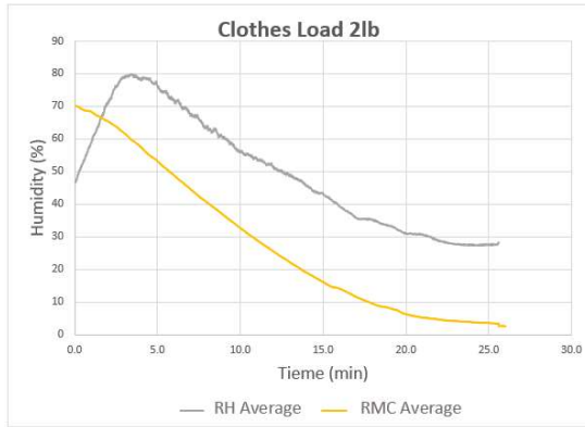
Fig. 1. Trend of RH average and RMC average during drying cycles for loads of 2 lb.
