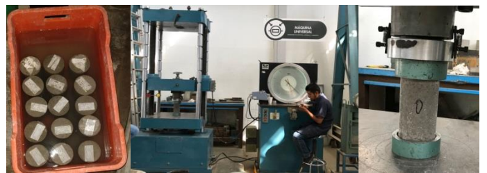
Figure 3. A) Curing of specimens B) Universal machine C) Cylinder test.
