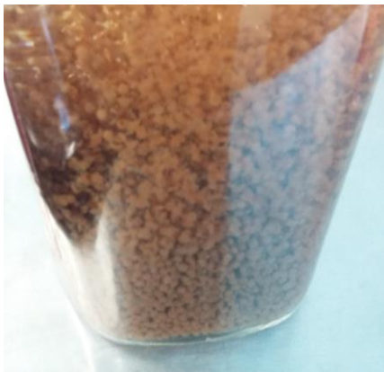
Fig. 2. Spheres of Chitosan-QGMA with magnetite nanoparticles.
