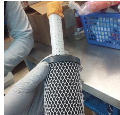
Fig. 3. Filter with pheres of Chitosan-QGMA with magnetite nanoparticles and activated carbon.
