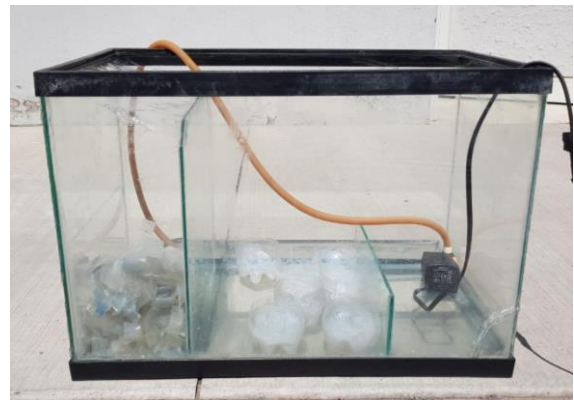
Fig. 1. Side view of prototype of rainwater treatment system.
