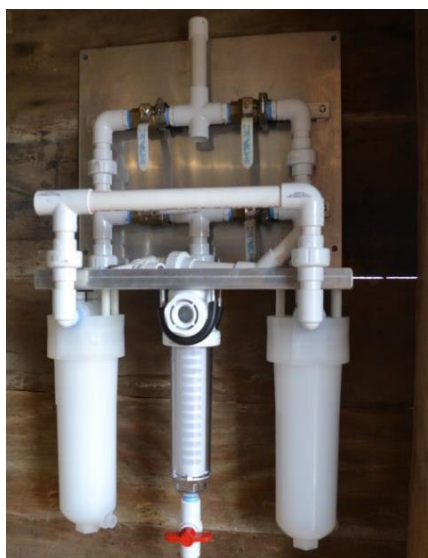
Fig. 2. Second stage: pathogen removal through hollow membrane filters.
