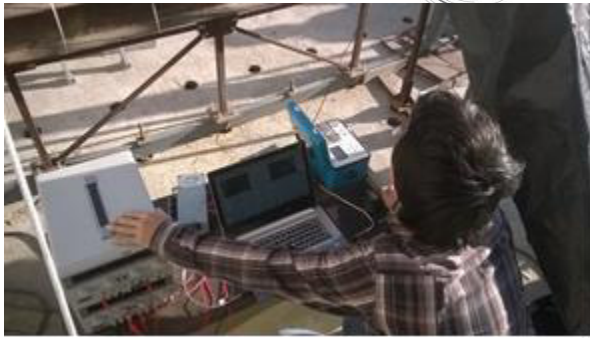
Image XVI. Instrumentation complements for the measurement of applied load and displacements.
