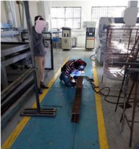
Image XI. Welding for IPR profiles at CEDIT.
