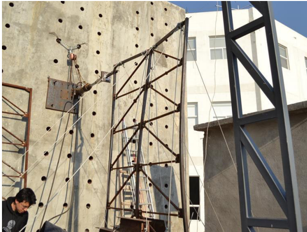
Image XX. Single panel system completely loaded with a side load of 2.70 tons on average. (5).
