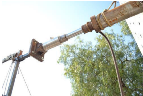
Image XVII. Connection of the piston to the lightweight panel.
