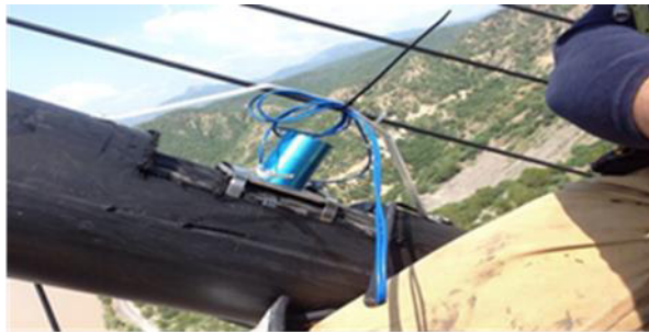
Fig.4. Accelerometer in cable
