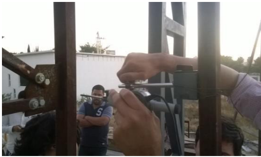
Image XXIII. Placement of micrometer to column to measure displacements outside the plane of the second panel.
