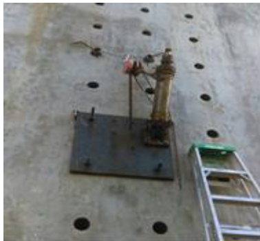
Image VII. Reaction wall loading piston.
