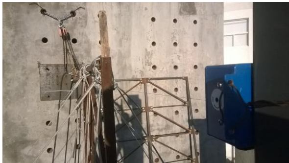
Image XVIII. Micrometer of thread fixed to the auxiliary structure.
