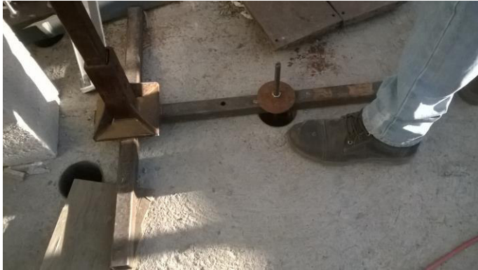
Image XXII. Fixed base to the reaction slab for secondary micrometer.
